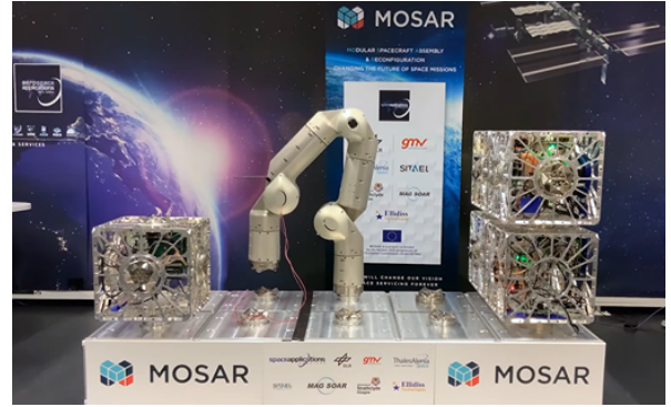
Fig. 1: Walking Manipulator (WM) for performing loco-manipulation tasks on a modular satellite.
