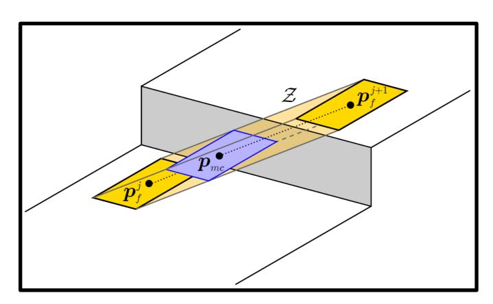
to avoid nonlinearities, we employ a moving constraint: the ZMP must belong to a fixed-shape region (the footprint) which slides between consecutive footsteps during double support, and coincides with a footstep during single support
