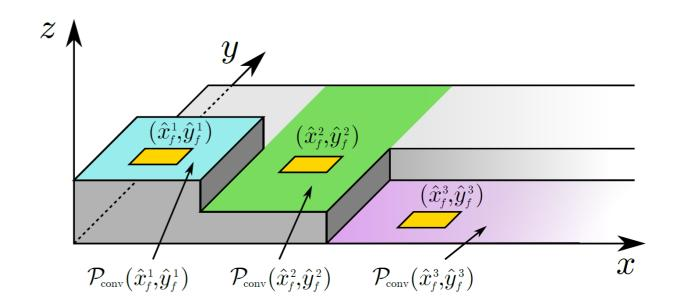
• **kinematic constraint**: ensures that footsteps are placed so as to be kinematically realizable by the robot
