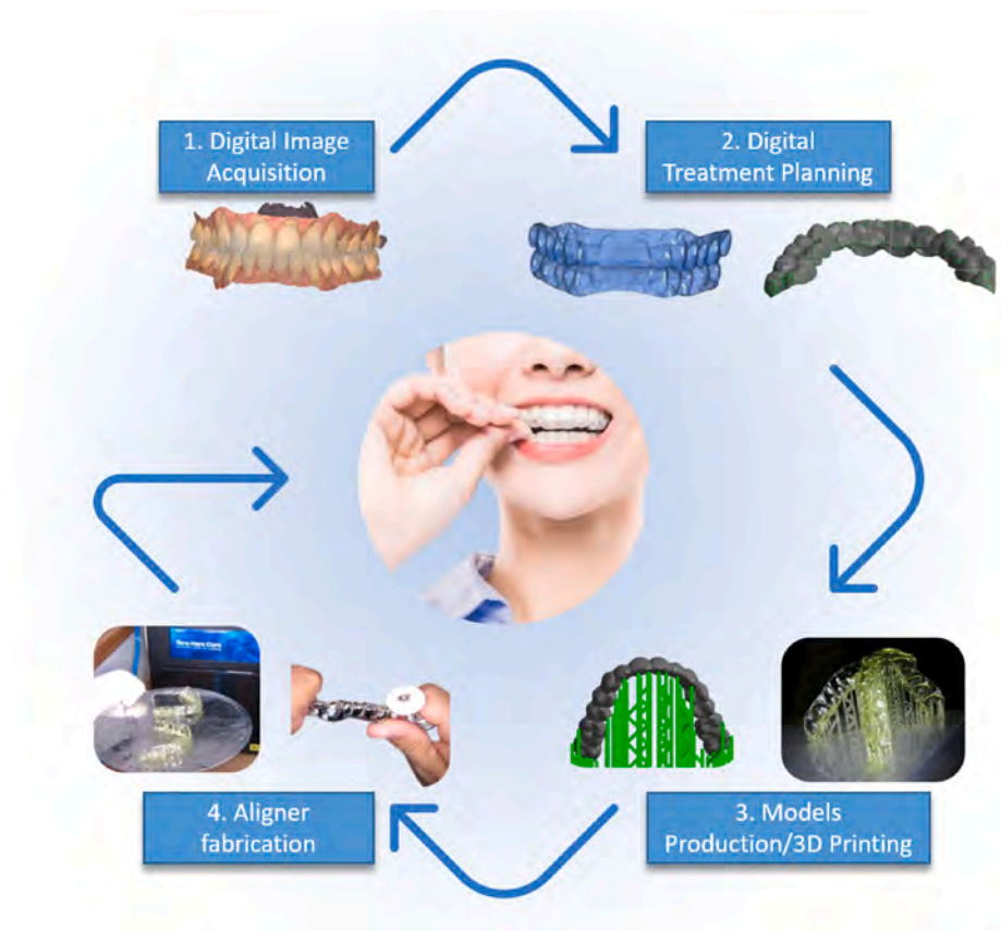
Fig. 2. Stepwise fabrication process of 3D direct printed clear aligners.
