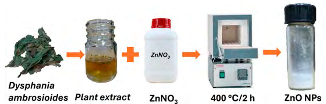
Figure 1. Green synthesis of the ZnO NPs.
