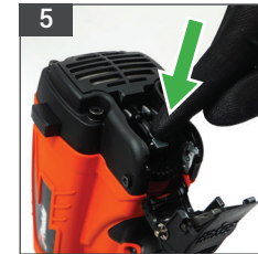
Lower fuel injection
